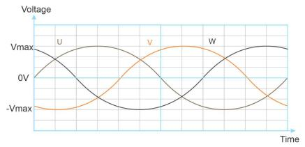
The signals are identical but 120 degrees apart. This is a hard signal to reproduce with power electronics. Something easy to produce might be like this:
