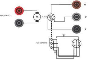
Unloaded, the brushless DC motor will generate 6V<sub>RMS</sub> between two phases at 2000 rpm.
