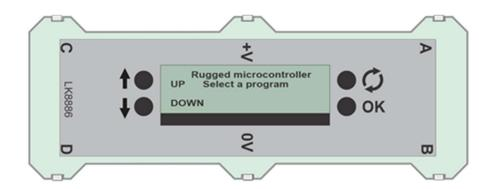
The LK8886 Micro ECU has six standard Locktronics legs that allow it to be inserted into the Locktronics base board.
